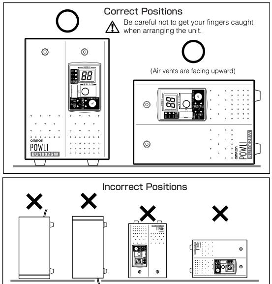
\* The feet can also be anchored to the floor with screws if you use BUP100S mounting brackets (sold separately). Refer to the BUP100S instruction manual for more details.
